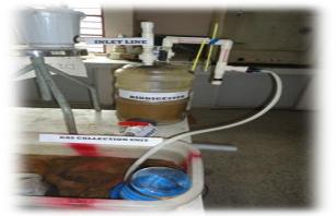
Figure 1. Set up of the fittings of the digester and operational digester 2.2 Designing procedure of the digester
